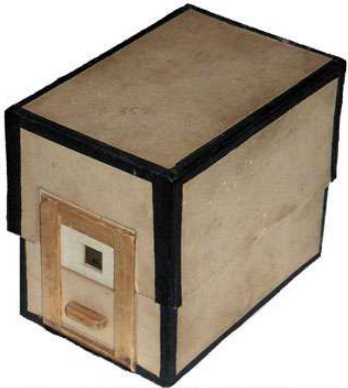
mat board pinhole camera, circa 1972
